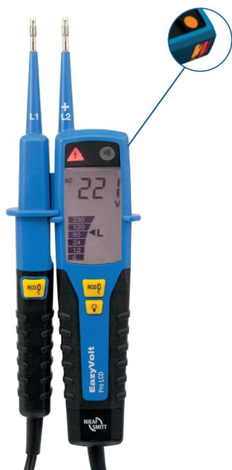
Thee EazyVolt Pro LCD is a reliable and safe 12-in-1 automatic voltage tester up to 1000 VAC and 1500 VDC, with the following functios:
