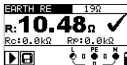
Figure 5.35: Example of earth resistance measurement result
