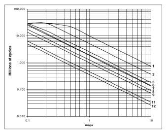
DC Current breaking capacity at L/R = 0
